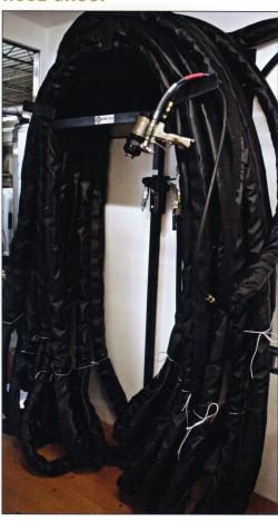
Our tough, hydronically heated hose group is wrapped with ballistic nylon to provide years of service in harsh jobsite conditions.
