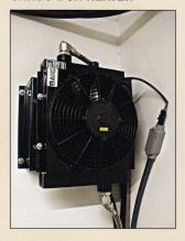
An optional Cargo Box Heater utilizes waste heat from the air compressor to warm the inside of the rig during cold winter months, keeping foam material and supplies warm inside the rig.
