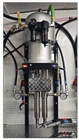
Our high performance, rugged Graco proportioning pump can deliver material up to 6 gpm, enough to supply two separate hose groups spraying simultaneously.
