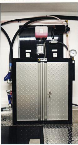
The USS proprietary design utilizes waste heat from our Kubota 3-cylinder engine to hydronically heat the hose and material. Material is heated prior to the proportioner pump for more balanced viscosities and better yields.
