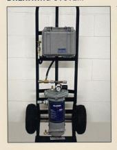
The integrated supplied air breathing system can provide breathable air to 4 workers simultaneously. An optional chiller can provide conditioned air to workers' hoods/masks to provide relief during summer months.
