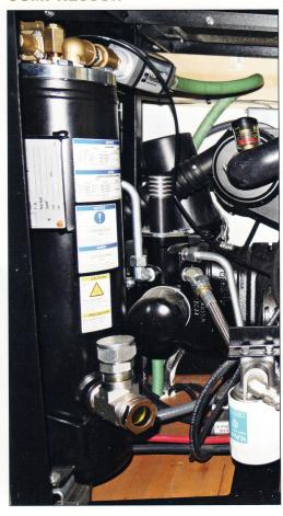
Our high volume, 92 CFM screw compressor powers the proportioner pump, transfer pumps, B-side barrel mixer (if required), breathing system for up to 4 workers, as well as an auxiliary air line for the workbench area.
